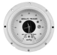
For routine test, laboratory, and production uses, this gauge gives accuracy and compact size. Its mechanism is sensitive yet rugged. And it offers high accuracy at low cost. Available in ten standard ranges, the Series 300 is convenient to use. Absolute pressure is applied to the case and readout is direct, without barometric or temperature corrections. Readings are referenced to zero absolute.
